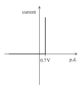
(a) Describe how the current through this diode varies for positive p.d.s and negative p.d.s.
