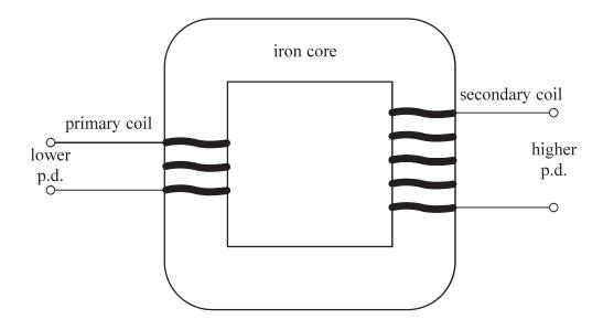
A step-up transformer is used to convert a lower p.d. to a higher p.d. An alternating p.d. is applied to the primary coil.
