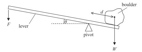
The centre of gravity of the boulder is a distance d from the pivot. The angle of the lever to the horizontal is  $\theta$ .
