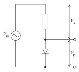
The p.d. across the resistor is  $V_{\rm R}$  and the p.d. across the diode is  $V_{\rm D}$ .  $V_{\rm D}$  is the output.
